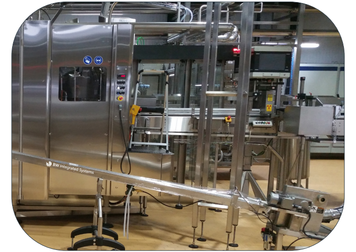
Fleetwood Manual Can Lid Feeder with LLV Low Level V-Tray in production
